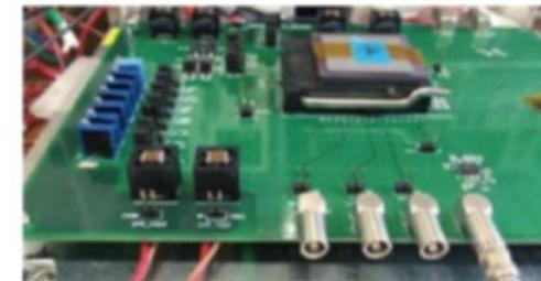
Multiple scattering at the slave DAQ board, a socket, and a ceramic package for SOFIST are causes of coarse spatial resolution.
