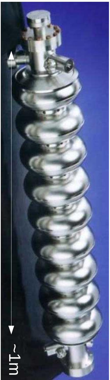
Niobium 1.3 GHz superconducting accelerating structures
