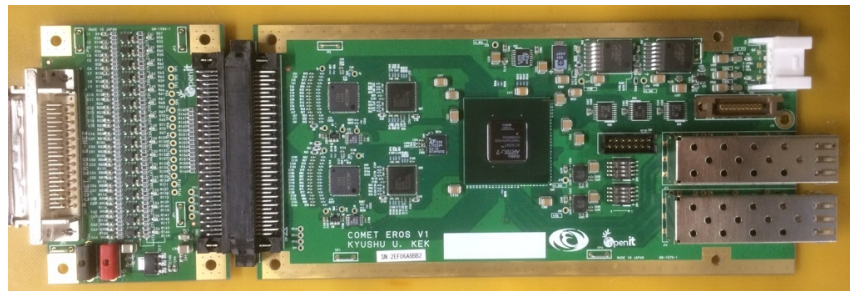
Figure 4.13: Waveform digitizer board for the ECAL, EROS. The mezzanine board on the left side converts the input differential waveforms into single-end waveforms.
