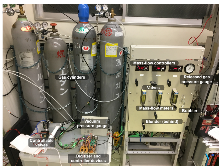
Figure 3.12: Prototype of gas and vacuum systems. The right panel contains all items used for controlling, mixing, and monitoring the gas flows. The digitizer and controller devices digitize the values monitored by the mass-flow controllers and vacuum pressure gauge, send them to the DAQ computer, and control the valves to open and close the gas-flow line.
