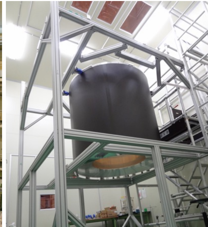
2015 Outer structure was transported to a KEK assembly hall, and set on a wire stringing cradle.
