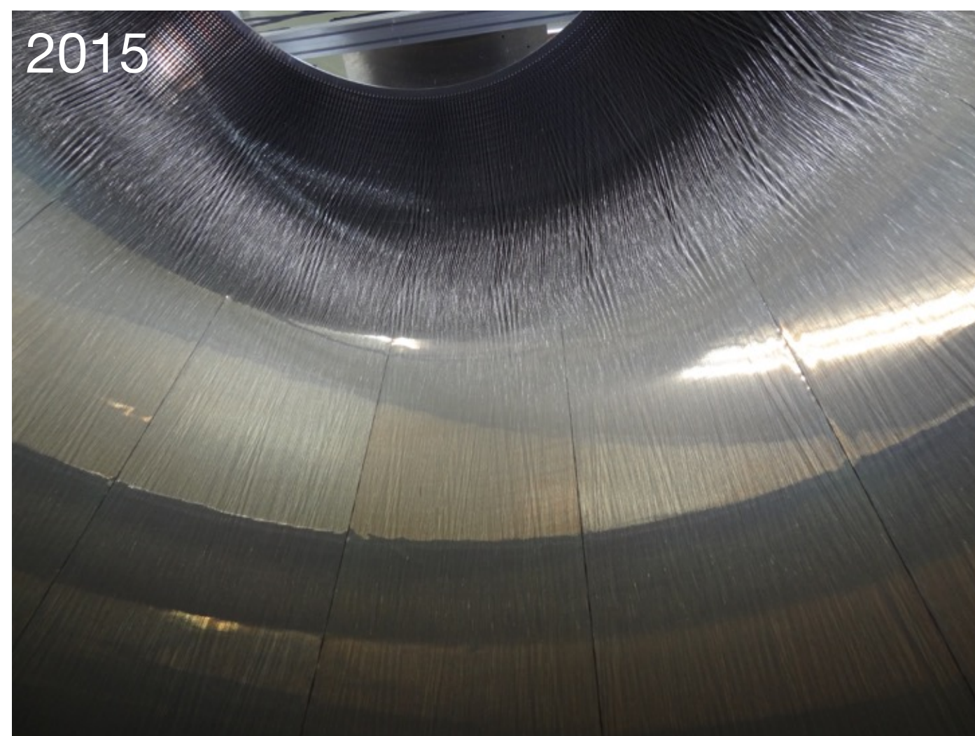
2015 Wire stringing and tension measurement for 19,548 wires were carried out in a half year.
